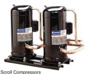
The compressor is the heart of a chiller's refrigeration cooling system. The compressor removes the refrigerant vapor from the evaporator to a point where the desired process fluid set point can be maintained and it raises the pressure of the refrigerant vapor to a level high enough so that the available condensing medium can effectively remove the process heat.
